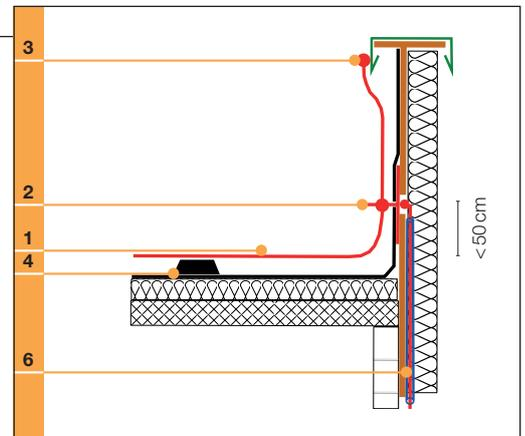
Concrete parapet with drain embedded in concrete.
