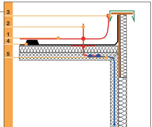
Wooden parapet with concealed drain.
