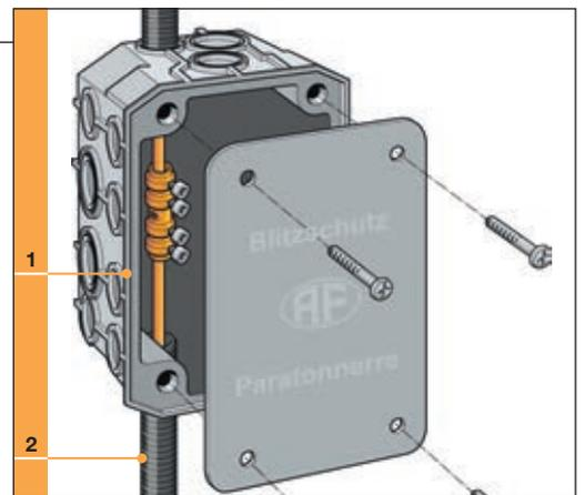
**Artificial Conductors in the Back Ventilation**
