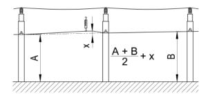
When replacing an existing section insulator measure the height of the contact wire at masts A and B. Calculate the average value. The hogging value should be minimun x = 70 mm.
