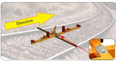
Place the JIG in a user-defined installation position. Adjust the level gauge.
